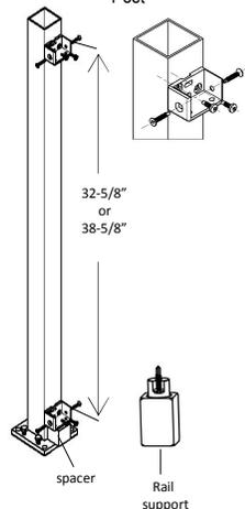
4. Fasten rail support to bottom side of bottom rail by inserting pan head self-tapping screw (provided) through center of threaded portion of support. This applies to all sections over 6ft long.
