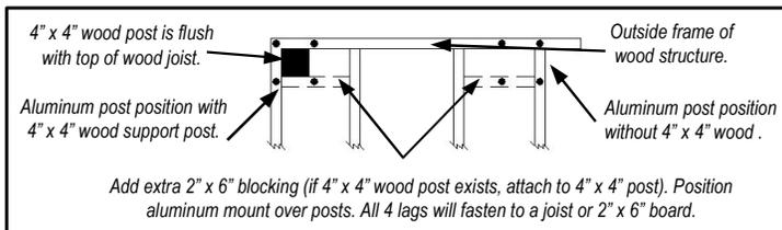
3. Use a 1/2" open end wrench to level aluminum post with the leveling bolts on the welded plate. **If using a 6" post attach one-piece flair now.**
