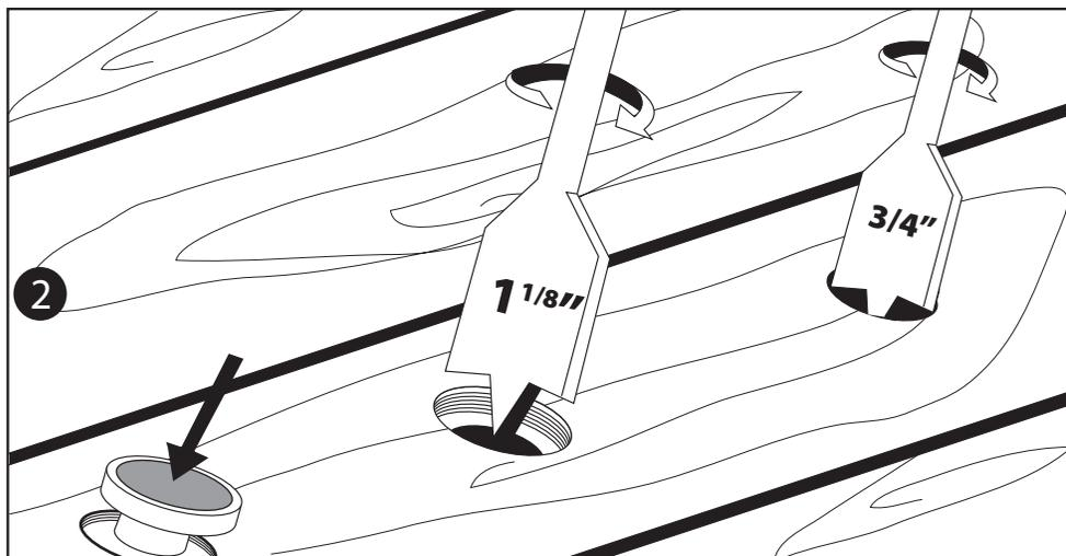
[ILLUS. 2] For each light, using a spade bit or forstner bit, drill a 1-1/8" hole approximately 1/4" deep. Check the depth by placing one of the LED lights upside down in the hole until the shoulder is flush with the decking surface. The bottom of your hole needs to be flat so the light lays in correctly. If necessary, use a chisel to scrape away excess material to flatten the bottom of the 1/4" hole.
