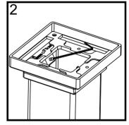
2. Place the Post Cap Base on the post. Using the supplied 2.5mm Allen Wrench tighten the two set screws. Adjust the screws to center and level the Post Cap on the post.
