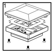
1. The following components are included with the FortressAccents 2" and 3" Flat Pyramid Caps: Post Cap, Post Cap Base, Light Slot Cover, 4 - Machine Screws, 2 - Hex Head Set Screws, and a 2.5mm Hex Wrench.
