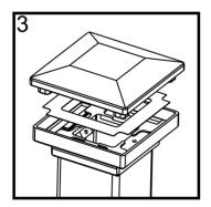
3. Place Light Slot Cover back onto Post Cap Base. Position Post Cap onto the Post Cap Base.
